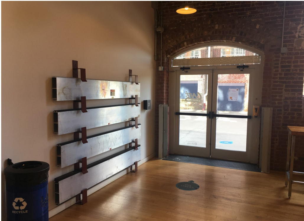
Flood shields for commercial buildings can be stored in the building as shown above and then deployed to protect the building during periods of high water (below) (New Bern, North Carolina, courtesy of the North Carolina State Historic Preservation Office).
